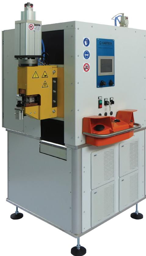
The machine GFA301000 has been developed to connect enameled wires and cables normally used in the electromechanical industry following the logic of a semiautomatic process combined with easiness of use, flexibility and high productivity so to get the best consistent and repetitive result.
